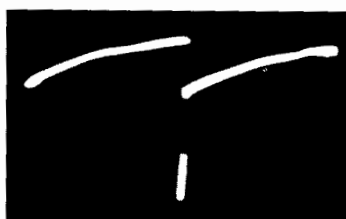
Fig. 12-7. Vertical deflection waveform from vertical output stage.
