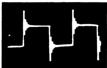
Fig. 10-7. Moderate ringing induced by application of square waves.
